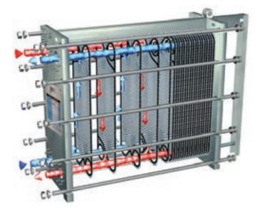
The arrangement of the plates creates two separate channel systems, enabling the two media to flow past and between each other without physical contact, leaving the exchanger again via connections in the pressure plates. Plate with different patterns can be mixed in the heat exchanger in order to achieve optimum efficiency at a given pressure drop.
