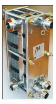
JeoTes™ plate heat exchanger is designed as single side flow. Flow passages can be formed by rotating the same plate 180°and arranging in a row. Consecutive plates are completely locked each other with an interlocking mechanism. The free bearing and the plates' easy moving in this bearing help the PHE to be tightened to an appropriate position. All bolts are covered with high-strength galvanization
