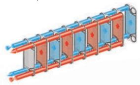
By install-ing special distribution plates in the plate pack, the media can be conducted several times through the flow channel.
