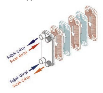
Different from the gasket seal type, brazing type uses soldering material, like copper or nickel depending on the application, to seal the exchanger. By applying high temperature in the vacuum environment at the manu–facturing process, it melts down the soldering material to form the seal between each plate.
